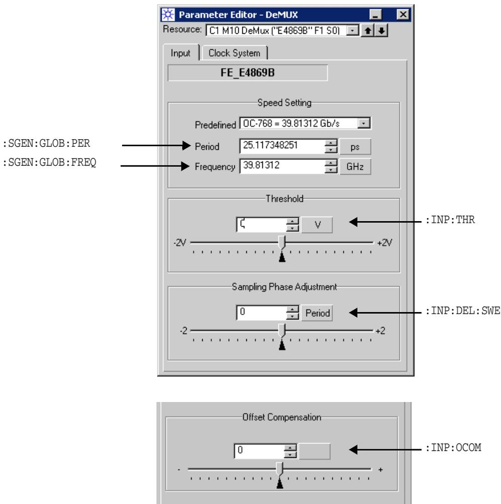
The following figure shows the clock system commands in the ParBERT user interface for a MUX module:
