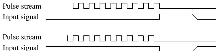
**NOTE** IMMEDIATE and START are always supported, GATED and STOP are only supported for E4832A modules.
