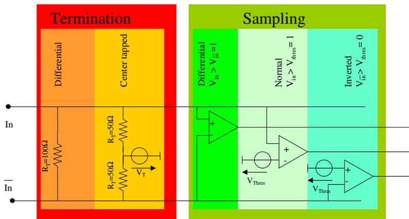
In NORMal and INVerted operation (“:INPut:IMPedance[:INTernal]” on page 252 and “:INPut:TVOLTage” on page 250) specify the termination of the input.
