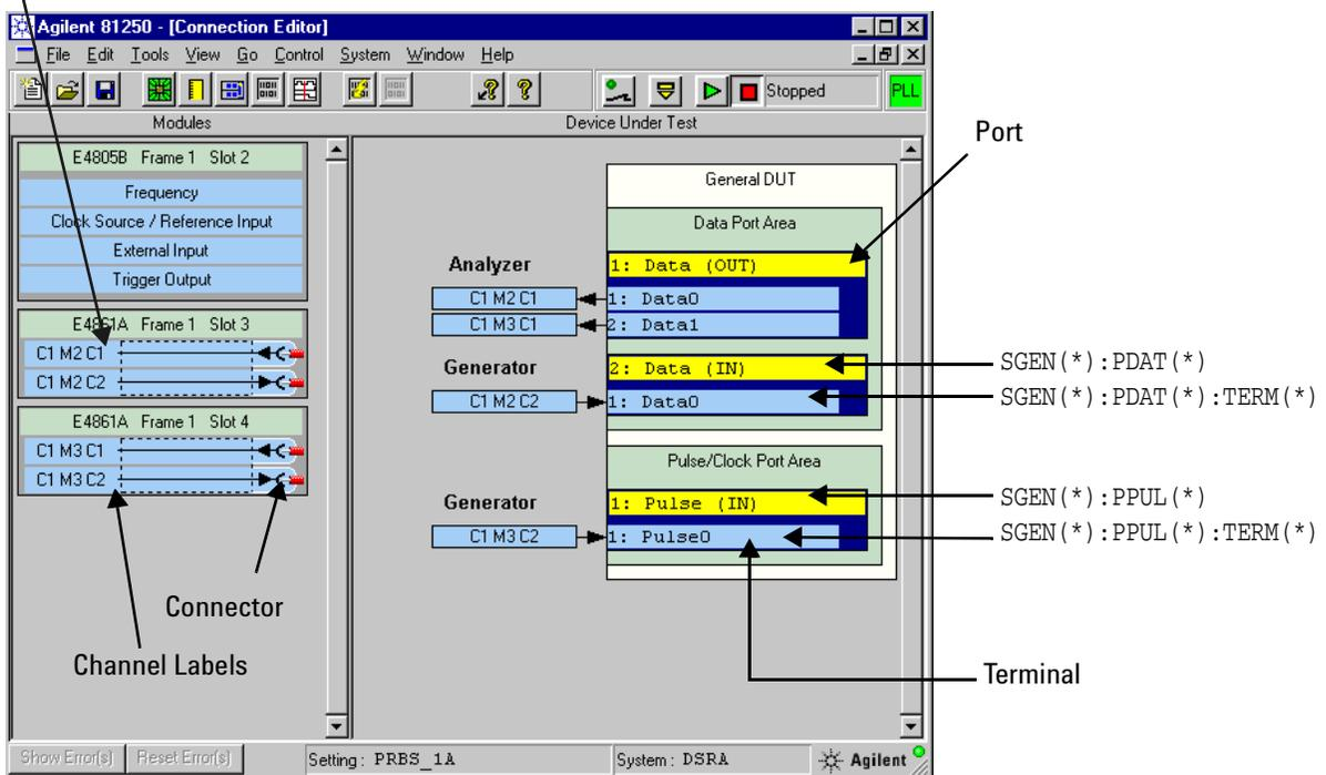
**Typical 43.2Gbit Analyzer Commands** The following figure shows some typical commands and their corresponding elements for a 43.2Gbit data analyzer system in the Agilent 81250 user interface:
