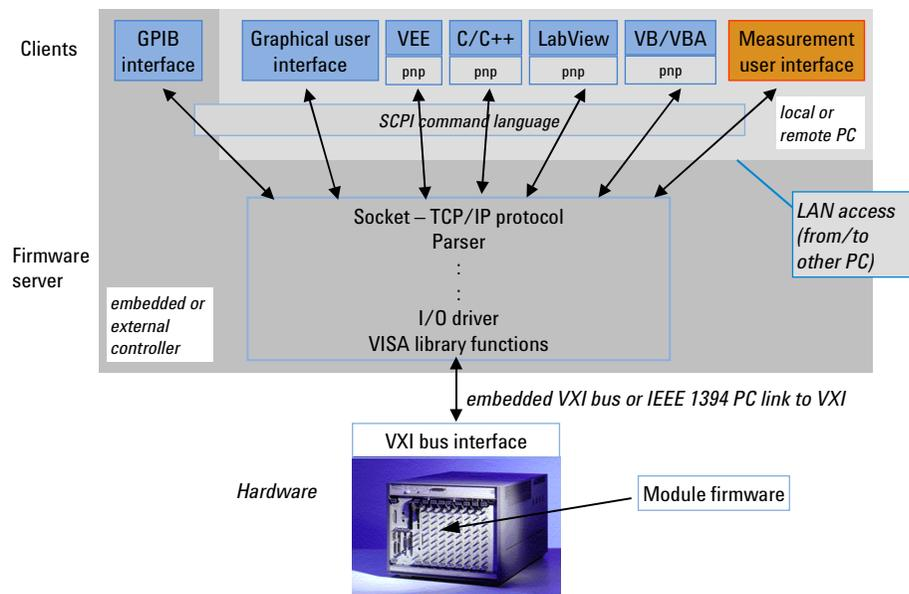
**Firmware Server and SCPI Commands** The user interface communicates with the firmware using the SCPI language. It implements a client-server architecture, allowing multiple clients to connect simultaneously.
