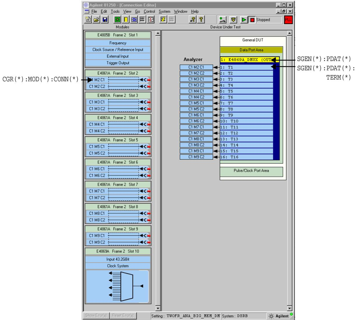
**Typical 43.2Gbit Generator Commands** The following figure shows some typical commands and their corresponding elements for a 43.2Gbit data generator system in the Agilent 81250 user interface:
