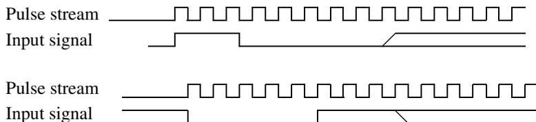
**...:SOUR:STOPsignal** The pulse stream (sequence) is stopped as soon as a stop signal exceeds the input threshold. The sequence can be stopped by a positive or negative input signal depending on the parameter set. All these modes are active if the system is started manually or started by a remote command.
