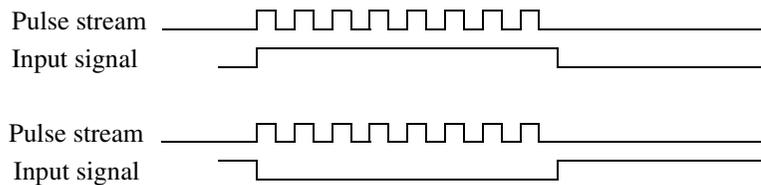
**...:SOUR:STARTsignal** A pulse stream (sequence) is generated as soon as a start signal exceeds the input threshold. A sequence can be started by a positive or a negative input signal depending on the parameter set.
