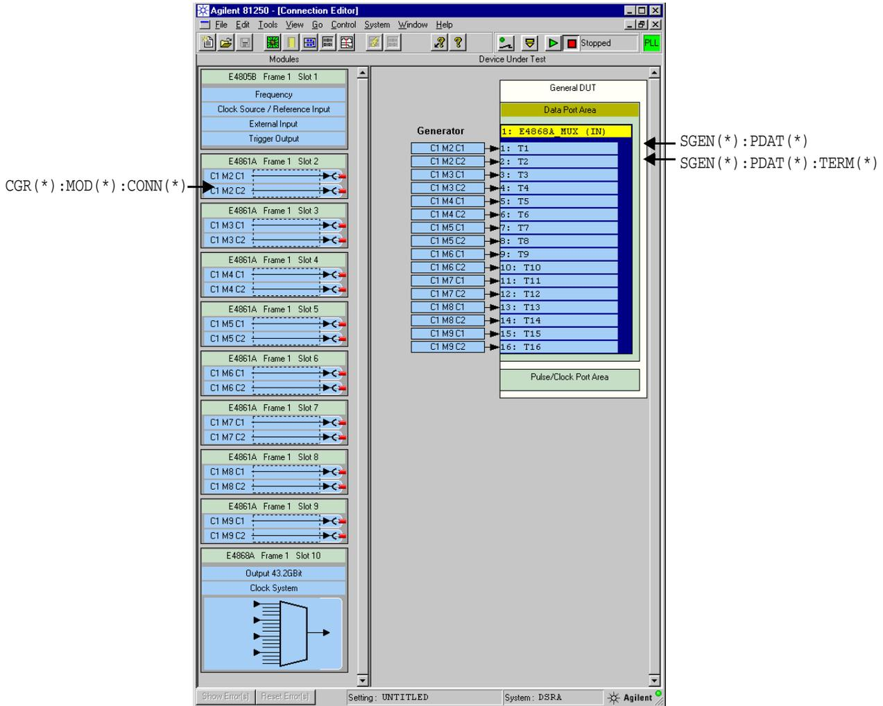
**Data ports and pulse ports** These figures also show how you can distinguish between data ports (:PDATa(\*):) and pulse ports (:PPULSe(\*):) on command level.
